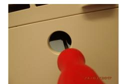
Take a screwdriver to help and clean the water outlet by twisting. Small tip: you can wrap a thin cleaning cloth around the screwdrive
